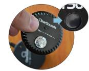
**STEP 3:** Scroll through the four levels of audio sensitivity by pressing and releasing the MMFB until you reach your desired level.
