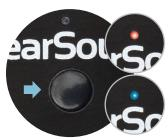
**STEP 2:** Quickly pair and connect the QT4 Mic: On the Mic, press and hold MMFB until light flashes red and blue.
