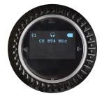
**STEP 3:** The Quattro 4.0 announces "Paired," and then "Device (number) connected." "CS QT4 Mic" appears on screen.
