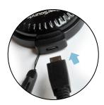
STEP 3: Plug the USB cable into the charging jack on the clip.
