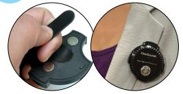
**OPTION 1:** On Clothing- Attach it to the speaker's clothing using the metal plate. For optimum performance, place the clip as close to the speaker's mouth as possible.
